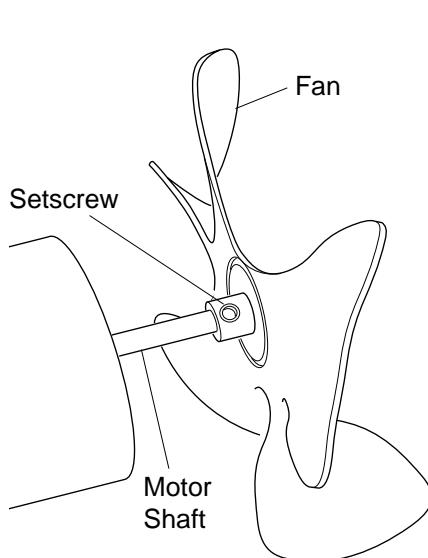
**Figure 17 - Fan, Motor Shaft, and Setscrew Location**
