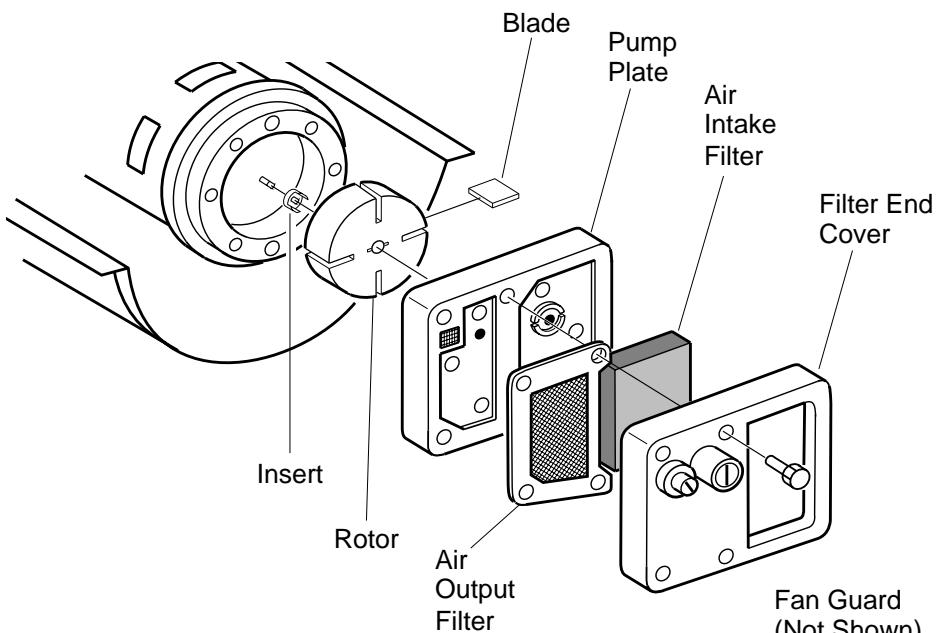
**Figure 14 - Rotor Location**
