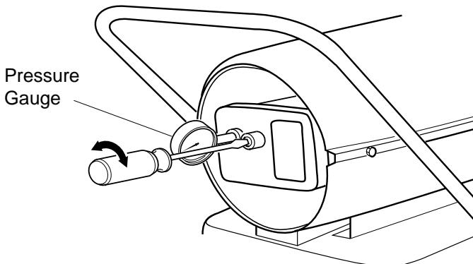
Figure 11 - Adjusting Pump Pressure
