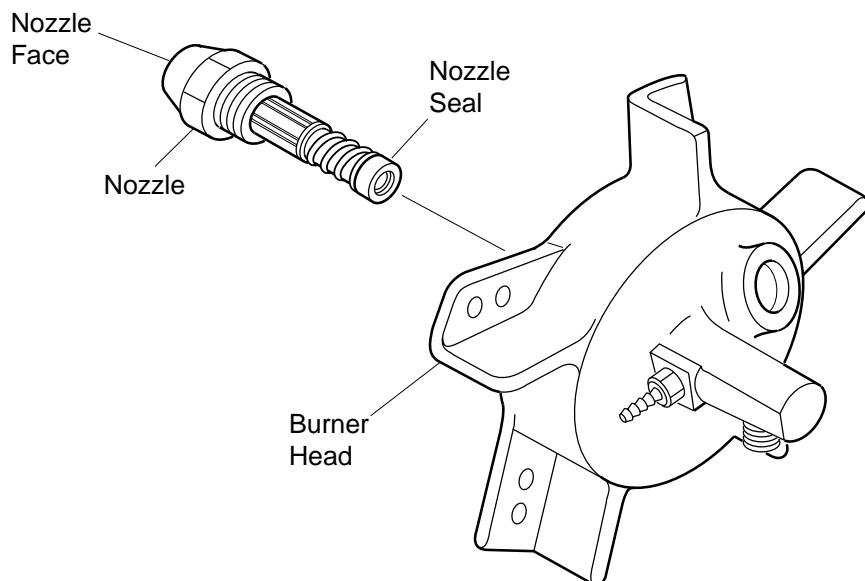
**Figure 13 - Removing Nozzle**
