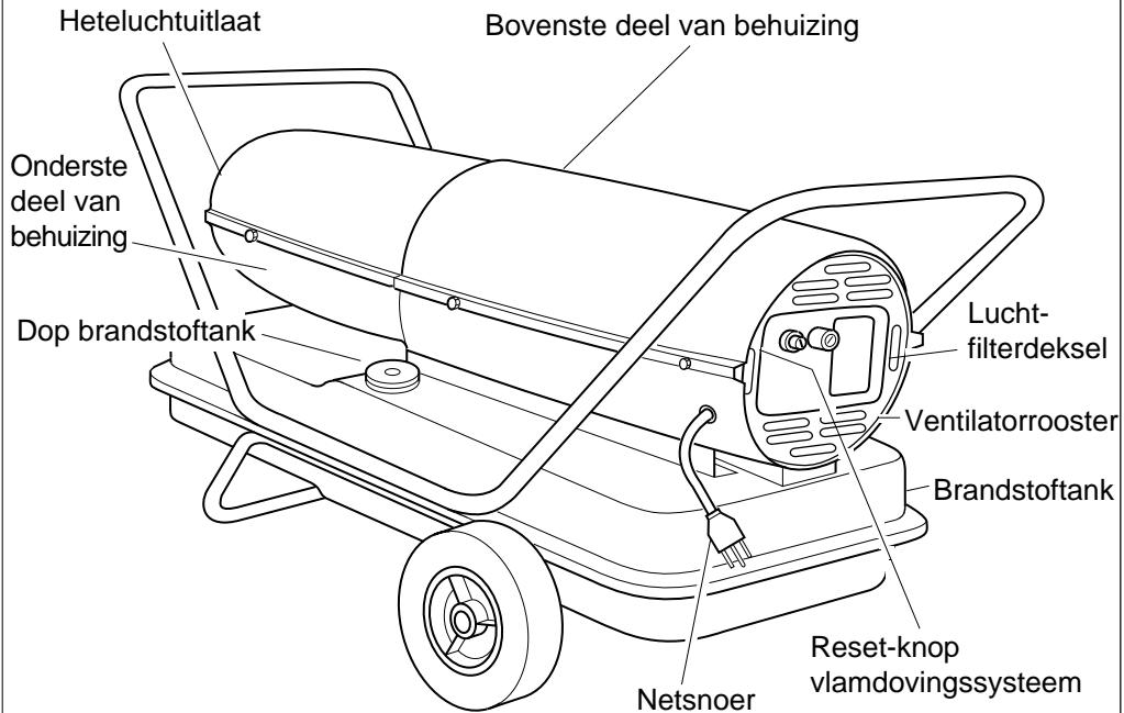
*Figuur 1 - Model 44 kW (150,000 BTU/Hr)*
