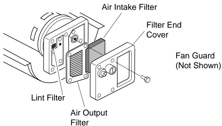
**Figure 9 - Air Output, Air Intake, and Lint Filters**
