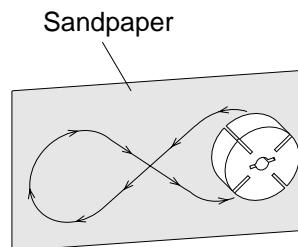
**Figure 16 - Sanding Rotor**
