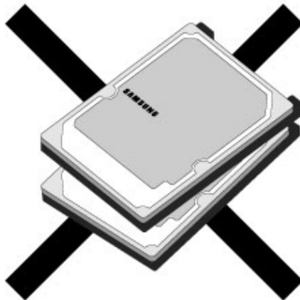
Fig. 9-3: HDD handling guide -Do Not Stack!
