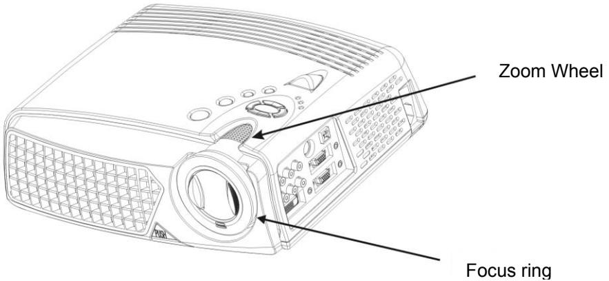
You can adjust the zoom ring to magnify or minify the image. Rotate counterclockwise to magnify the image. Rotate clockwise to minify the image. To adjust the focus, please rotate the focus ring to obtain the best focus. The focus distance of this projector is 1.4~12 meter.
