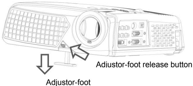
To adjust the tilt angle of the projector
