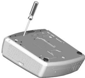
Remove the three lamp module retaining screws, unsnap the lamp removal handle to change the lamp module.
