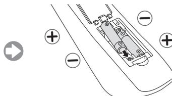
Insert two **AAA/R6** or equivalent type batteries inside. Place the batteries in the right directions.
