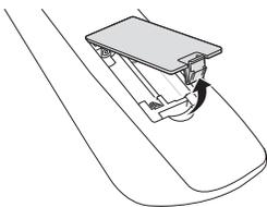
Remove the battery cover located on the back of the handset by gently pulling downwards from the indicated part.
