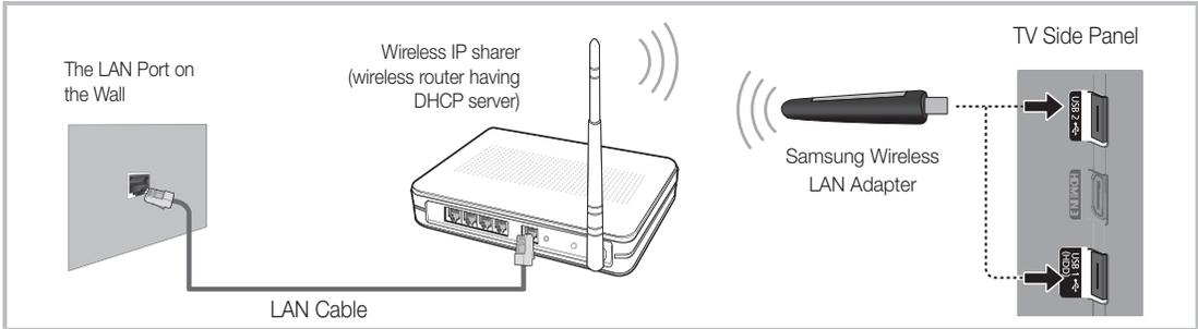
Samsung's Wireless LAN adapter is sold separately and is offered by select retailers, Ecommerce sites and Samsungparts.com. Samsung's Wireless LAN adapter supports the IEEE 802.11a/b/g and n communication protocols. Samsung recommends using IEEE 802.11n. When you play the video over a IEEE 802.11b/g connection, the video may not play smoothly.
