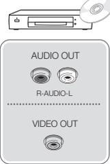
**Using a Component (up to 1080p) or Audio/Video (480i only) and Scart Cable**
