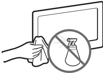
Do not spray water or a cleaning agent directly onto the product. Any liquid that goes into the product may cause a failure, fire, or electric shock.
