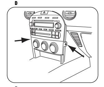
Pull radio/climate control panel out, disconnect plugs and remove. (Figure E)
