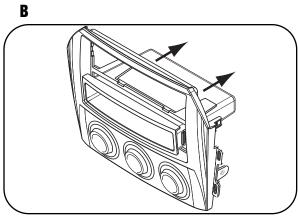
3 Slide the DIN cage into the Radio Housing and secure by bending the metal locking tabs down. (Figure C)
