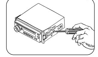
5 Snap the Trim plate into the Radio Housing. (Figure D)
