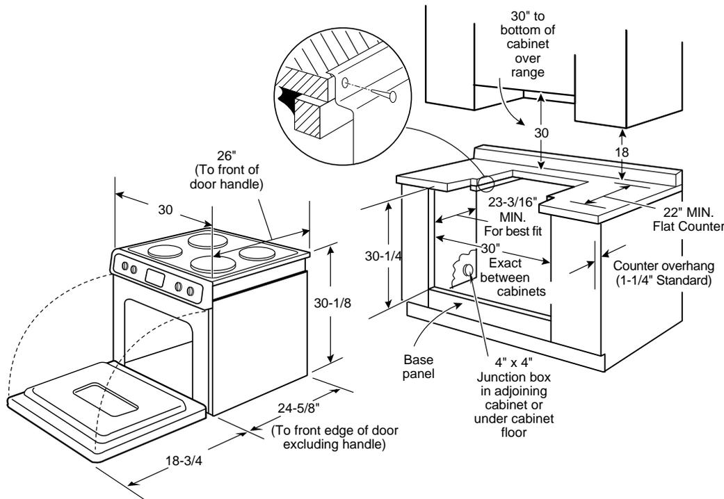
**Note:** Cabinets installed adjacent to drop-in ranges must have an adhesion spec of at least 194°
