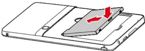
To remove the battery, do as the following figure.
