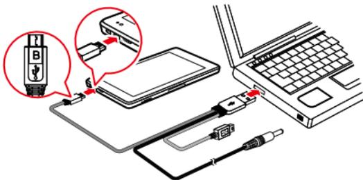
1. Use the USB cable that came with your Tablet to connect the Tablet to a USB port on your computer. The Tablet displays a notification indicating that the USB is connected.
