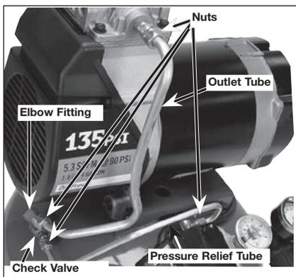
4. Using an adjustable wrench loosen pressure relief tube nut at air tank and pressure switch. Carefully move pressure relief tube away from check valve.
