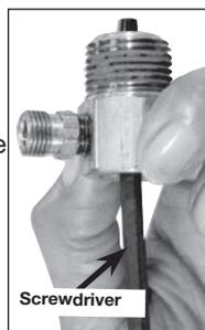
8. Clean or replace the check valve. A solvent, such as paint or varnish remover can be used to clean the check valve.
