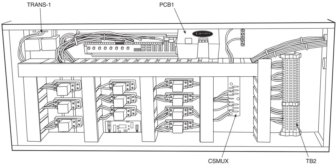
**Fig. 27 — Modular Unit VAV Control Panel**
