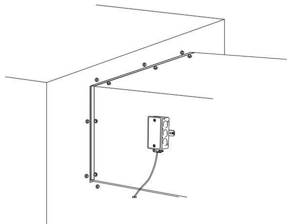
**Fig. 30 — Supply-Air Temperature Sensor Installation (Unit Discharge Location)**
