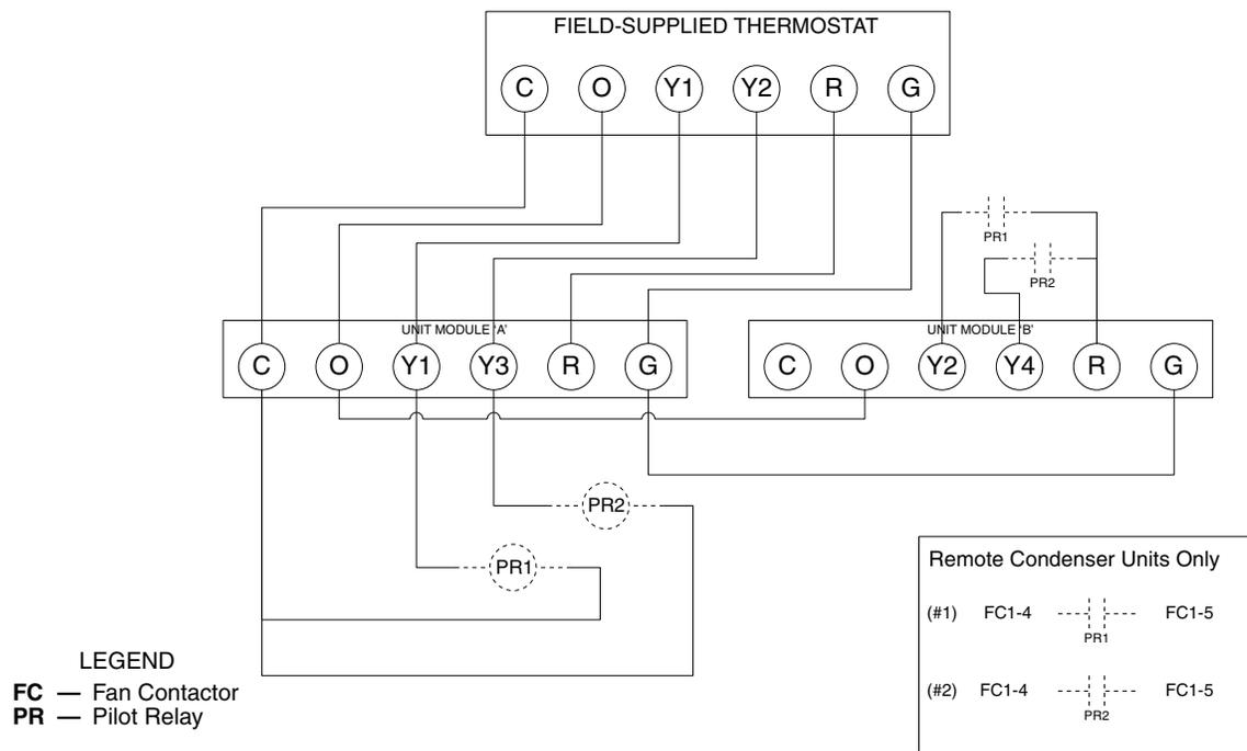
**Fig. 25 — Typical Wiring 40 to 60 Ton Units (Two-Stage Cooling)**
