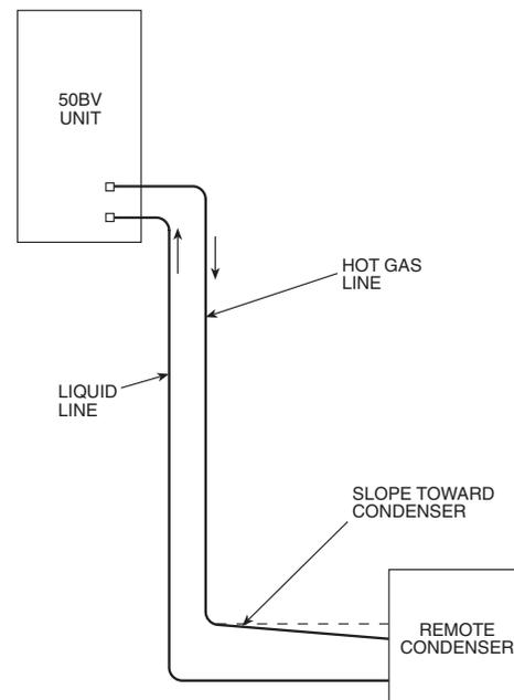
**Fig. 23 — System with Evaporator Above Condenser**
