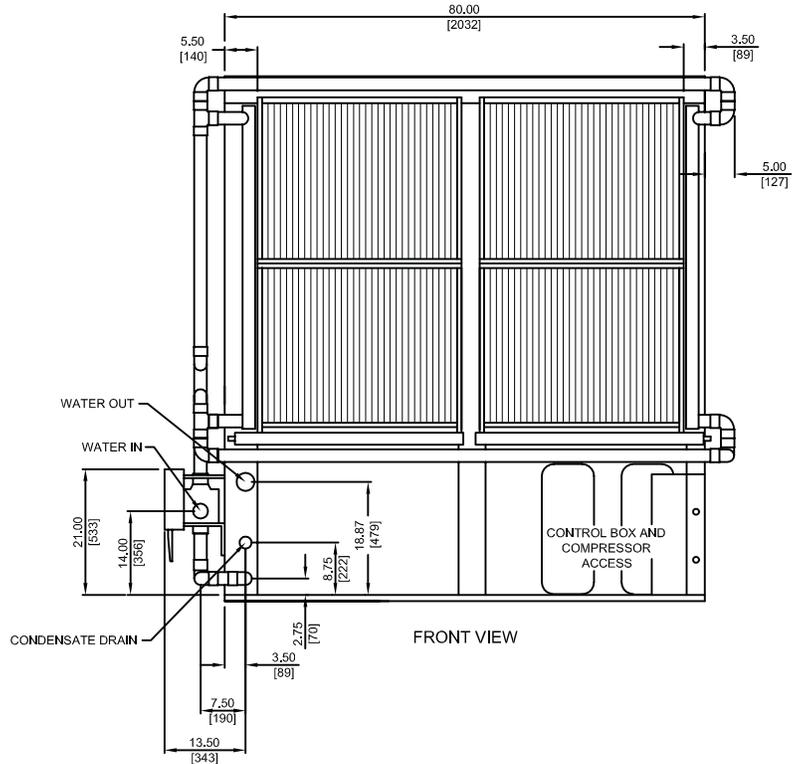
Fig. 13 — 50BVC,J,Q034 with Optional Waterside Economizer Dimensions
