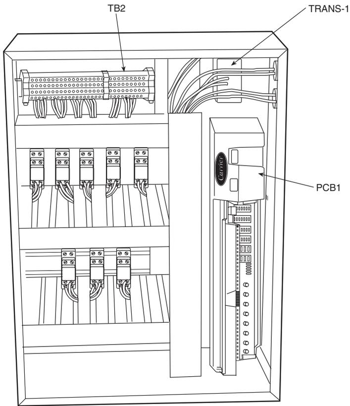
**Fig. 28 — Single-Piece Unit VAV Control Panel**
