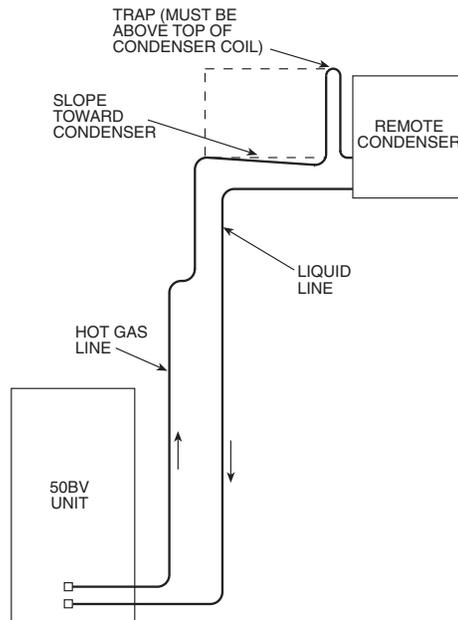
**Fig. 22 — System with Condenser Above Evaporator**
