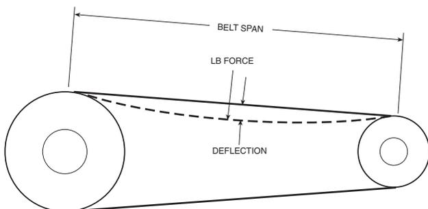
**Fig. 37 — Fan Belt Tension**
