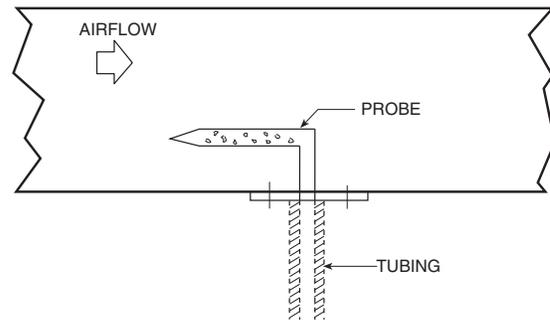
**Fig. 16 — Duct Static Pressure Probe (P/N 39EK20462)**
