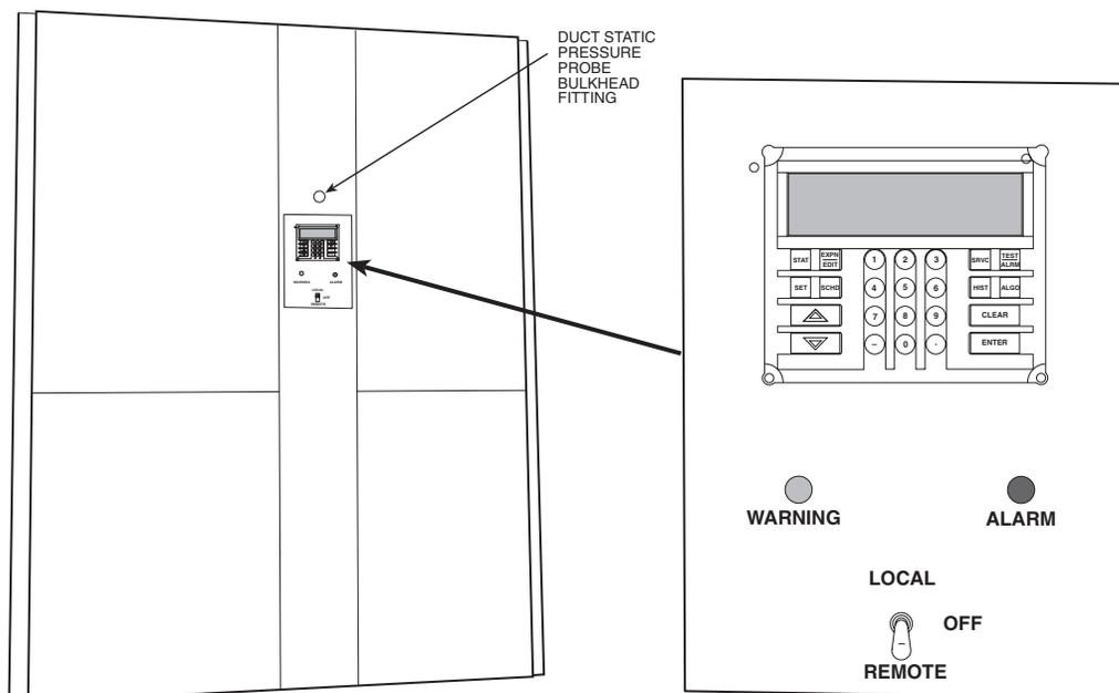
**Fig. 17 — Display Panel Location on Unit Front Panel**
