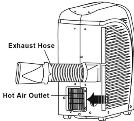
The hot exhaust air can be vented through the wall or out a window. If mounting in the wall, the height of the hole should be 14 1/4" to 60 5/8" (36cm to 150cm).
