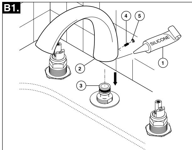
**NOTE: The deck and valve rough-in must be finished before installing the trim kit.**
