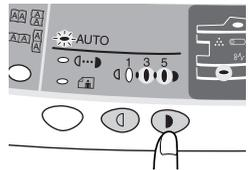
**5** Press the exposure selector key. The AUTO indicator will stop blinking and light up steadily.
