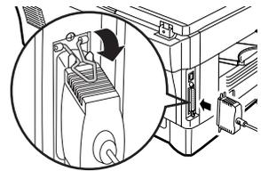
**4** Insert the other end of the cable into the interface connector of your computer.
