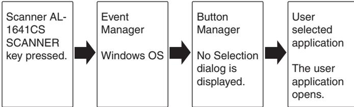
The settings for the Windows Event Manager for the SHARP AL-1641CS device allow the user to take advantage of the Sharp Button Manager to take control of events from Windows and send scanned images to any application that can be selected in Button Manager.
