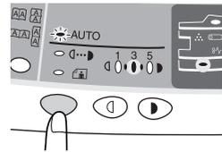
**4** Press the light (◀) or dark (▶) key to lighten or darken the automatic exposure level as desired. If exposure level 2 is selected, the two left-handmost indicators for that level will light up simultaneously. Also, if level 4 is selected, the two right-handmost indicators for that level will light up simultaneously.
