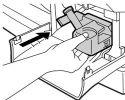
**4** Gently install the TD cartridge. To install the TD cartridge, see "INSTALLING THE TD CARTRIDGE" (p.10).
