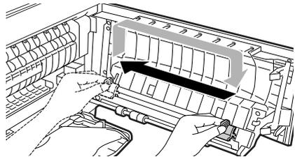
**4** Return the charger cleaner to its original position. Close the side cover by pressing the round projections near the side cover open button.
