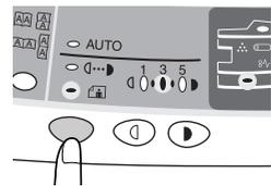
**3** Press and hold down the exposure mode selector key for approximately 5 seconds. The PHOTO (📷) indicator will go out and the AUTO indicator will begin to blink. One or two light and dark indicators corresponding to the automatic exposure level which has been selected will light up.
