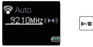
Each press of the button switches the tuning mode in order of "Auto" → "Manual" → "Preset".
