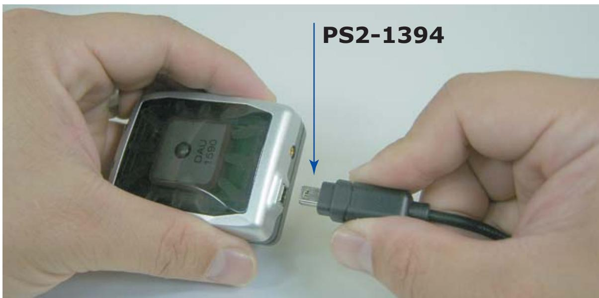
By connecting to different optional connecting cables, HI-406BT-C can be a wired PS/II GPS receiver and used with all kinds of mobile devices.
