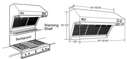
Each hood is shipped with a stainless steel backguard and a warming shelf. Hoods may be installed with the shelf or backguard alone, or with both as shown.
