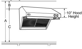
We recommend that the vent hood and decorative duct cover (if used) be on site before final framing and wall finishing. This will help to accurately locate studs, ductwork and electrical service.
