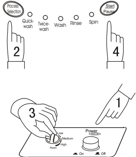
**1 Push the "Power " button to switch on the power**
