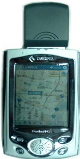
*Image 1: TN202 installed in PDA*
