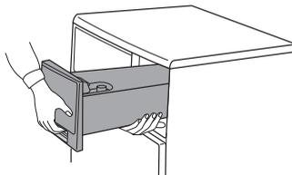
**☞** Push the cover of the condensate container to the side and pour-out the condensed water.
