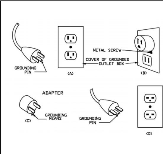
**WARNING:** This heater is for use on 120 volts. The cord has a plug as shown in A. An adapter as shown in C is available for connecting three-blade grounding-type plugs to two-slot receptacles. The grounding lug extending from the adapter must be connected to a permanent ground such as a properly grounded outlet box. The adapter should not be used if a three-slot grounded receptacle is available.
