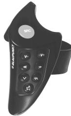
The RC 08 infrared remote-control permits operation of the chief functions from the steering wheel.
