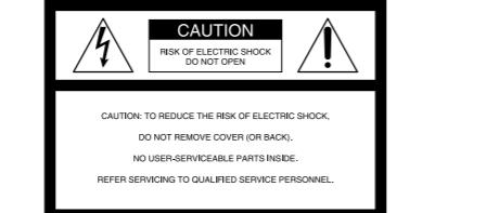
This symbol is intended to alert the user to the presence of uninsulated "dangerous voltage" within the product's enclosure that may be of sufficient magnitude to constitute a risk of electric shock to persons.
