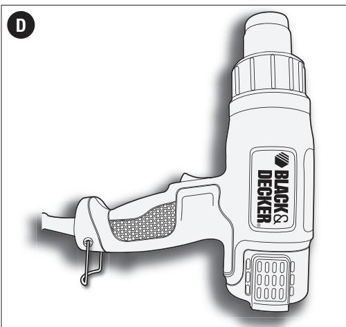
materials and soften or melt others. Avoid overheating adjacent flammable materials such as wood, insulation, electrical wiring jackets or plastic. Thaw only those metal pipe sections that are fully exposed. Do not attempt to thaw pipes that are inside walls, floors, ceilings, or otherwise enclosed. Do not attempt to thaw pipes that are wrapped in insulation.
