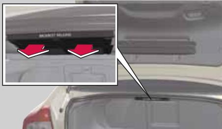
**Pull release handles separately** to fold left and/or right backrest.
