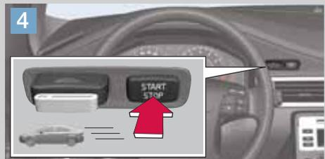
**Simply press START/STOP** button to start the engine.
