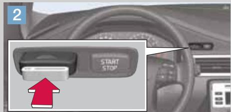
**Gently push the remote.** The remote ejects. Automatic transmission must be in position P.
