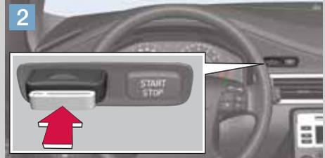
**Gently push the remote.** The remote is pulled into position.
