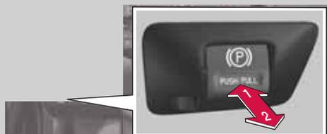
With a gear selected and accelerator pedal depressed the brake releases when you start driving.
