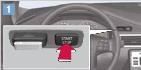
**Park the car and push Start/Stop** button to stop the engine.
