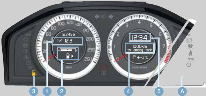
**1 Trip odometer.** To measure distance the car has two independent trip odometers T1 & T2 always running.
