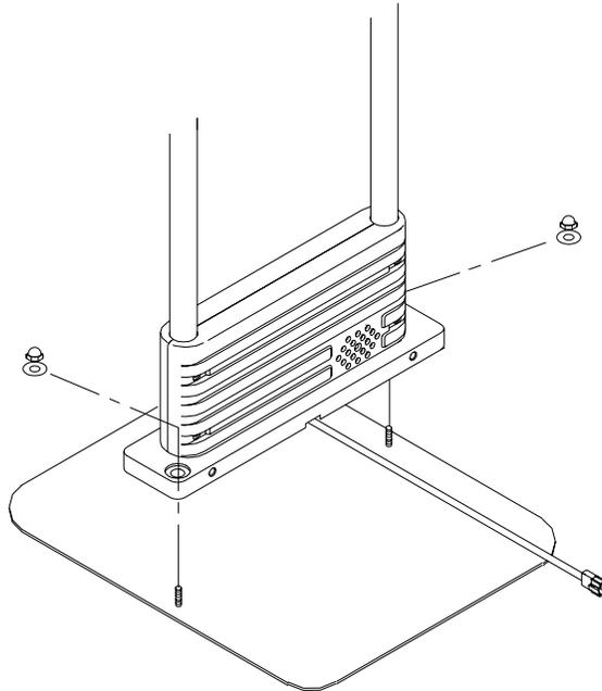
5. Connect the wire on the power supply to the power wire connected to the antenna. The wires will only connect in one direction.
