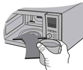
**6** Press the **STOP** button, and press the **START** button one time to set 30 seconds of cooking time. You will hear a BEEP each time you press the button. Your oven will start before you have finished the sixth press; don't worry this is normal.
