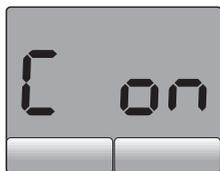
The same symbol will also be displayed whenever any button is pressed while the machine is child-locked. Child-proof lock lamp on the Programme follow-up indicator will light up when the child-proof lock is activated. To deactivate the child-proof lock, press the 1st and 2nd auxiliary function buttons for 3 sec. "C OFF" (Child-proof lock is deactivated) symbol appears on the screen.
