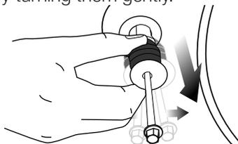
3. Fit the covers (supplied in the bag with the Operation Manual) into the holes on the rear panel. ("P")
