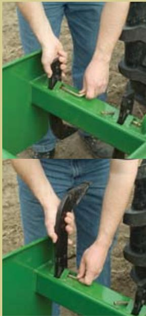
Choose from three scarifier depth adjustments to meet a variety of ground conditions. Adjustments are easy! Simply remove the steel pin, and raise or lower the scarifier to increase or decrease ground penetration. Scarifier shanks can be stored on the scarifier beam when using the box blade for other tasks.
