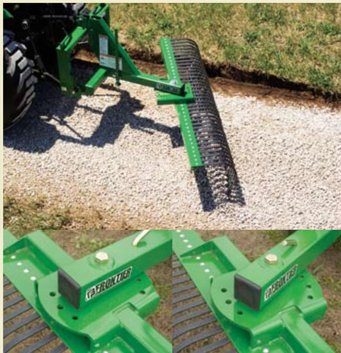
Achieve the desired raking profile by adjusting the tine beam in one of five different positions forward and three positions in reverse. Simply remove the steel pin and rotate the beam to the desired setting.
