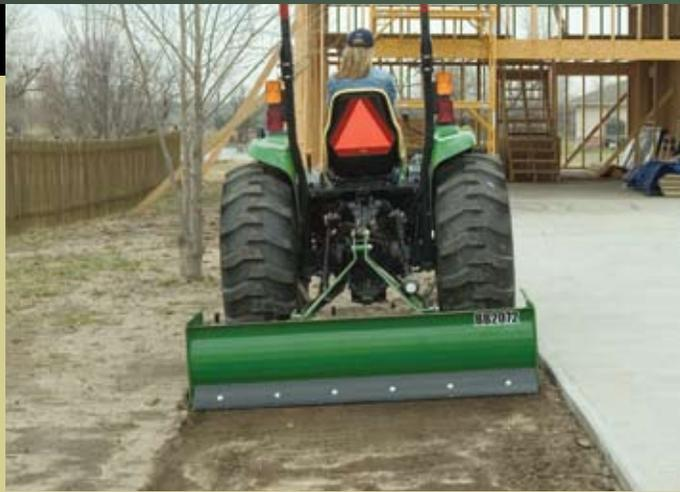
Heavy-duty, concave back plate with formed upper edge provides added rigidity and strength for trouble-free performance.
