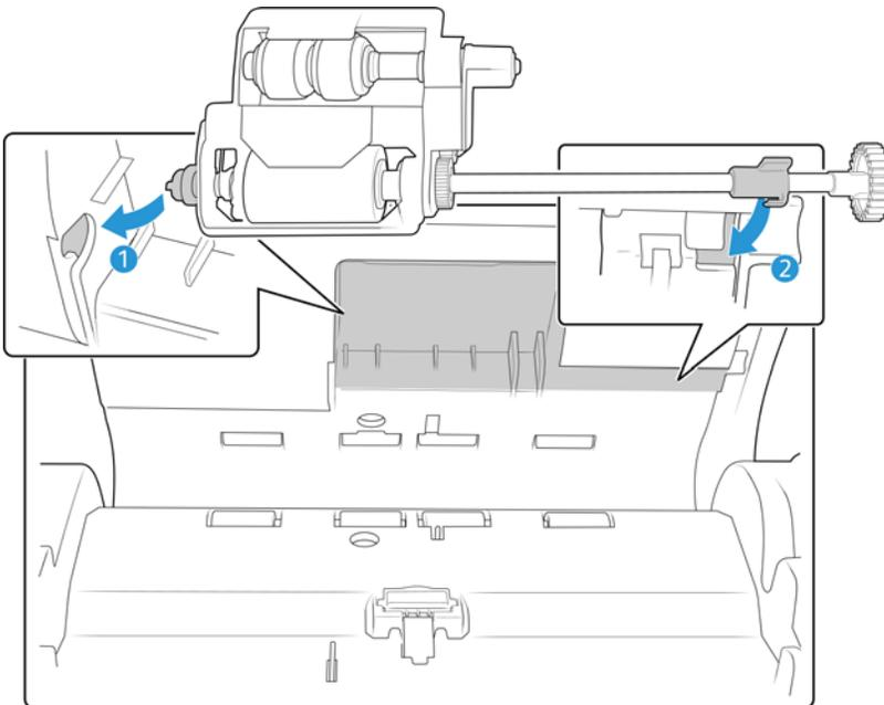
8. Align the tab on the lock flange with the slot in the scanner. Use the lever to rotate the locking tab into the slot in the scanner. Push on the lever until it clicks in place and locks the roller in the ADF door.
