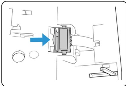
3. Lift the pad up and out of the scanner.
