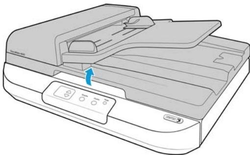
4. Remove any tape and protective foam from around or on the flatbed glass.
