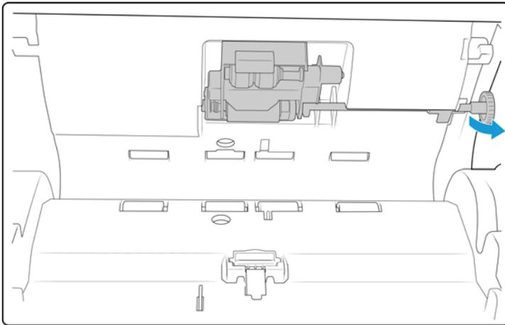
5. Before installing the new roller, clean any dust that may have gotten on it during shipping.
