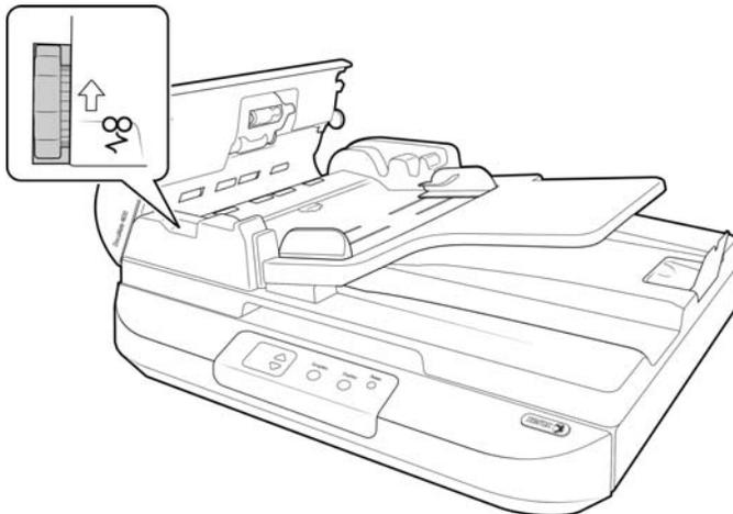
2. Close the Automatic Document Feeder cover when you are finished. Carefully press down on the ADF cover until it locks in place with a “click”.
