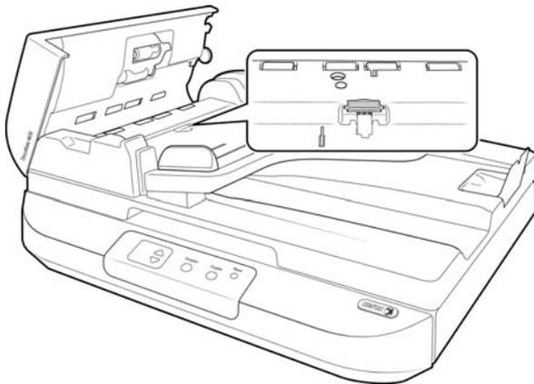
2. Squeeze the plastic clamp that holds the pad assembly in place.
