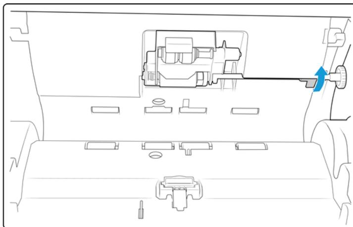
4. Remove the roller from the scanner and discard it, it cannot be repaired.
