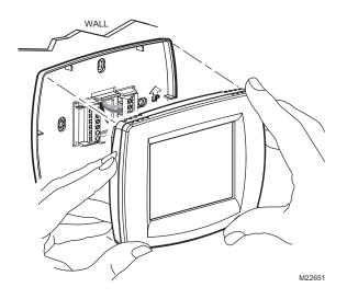
3. Remove the old batteries and insert three fresh AAA alkaline batteries, as marked on the comfort control.
