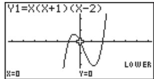
3. Use **◀** to move the pointer to the location where  $X = -1$ , and then press **EXE**. Next, use **▶** to move the pointer to the location where  $X = 0$ , and then press **EXE** to input the integration range, which becomes shaded on the display.
