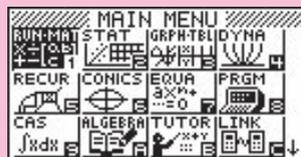
6. Use the cursor keys (▲, ▼, ◀, ▶) to select the **SYSTEM** icon and press **EXE**, then press **F2** (◀▶) to display the contrast adjustment screen.
