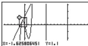
4. Press , and the enlarged area appears in the inactive (right side) screen.
