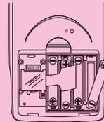
3. Remove the insulating sheet at the location marked "BACK UP" by pulling in the direction indicated by the arrow.
