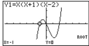
**Example 3:** Determine the area bounded by the origin and the  $X = -1$  root obtained for  $Y = X(X + 1)(X - 2)$
