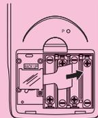
4. Replace the back cover, making sure that its tabs enter the holes marked ② and turn the calculator front side up. The calculator should automatically turn on power and perform the memory reset operation.
