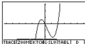
**Example 2:** To determine the roots of  $Y = X(X + 1)(X - 2)$
