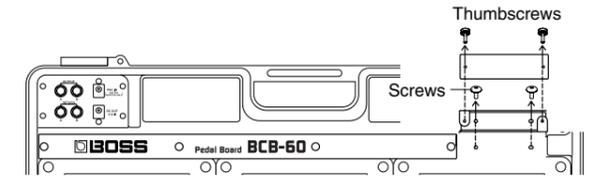
Attach the wah pedal as shown in the figure. Set the wah pedal's rubber feet in the depressions.
