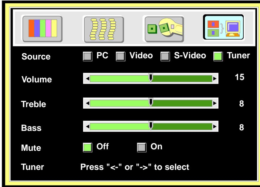
2. Use the Menu key on the control pad or remote control unit to scroll through the Tuner sub-menu.
