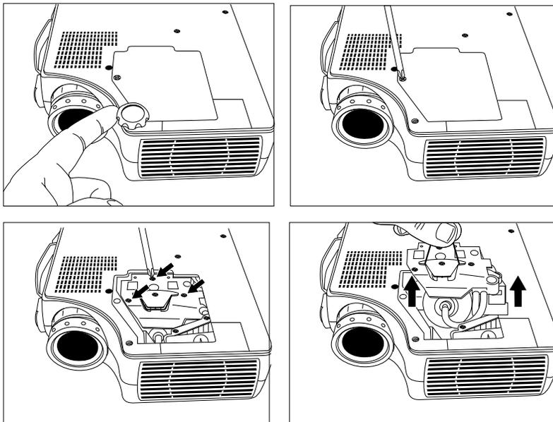
✓ *Note: For maximum lamp life, do not shock, handle or scratch the lamp glass when it is hot. Also, do not use an old or previously used lamp as a replacement lamp.*
