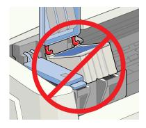
8. Press down the ink cartridge clamp until it locks in place. (The color clamp is a bit harder to close than the black clamp.)
