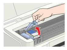
5. Lift the cartridge out of the printer and dispose of it carefully.
