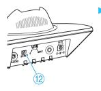
Set the ST/MO switch 12 on the transmitter to MO (mono).
