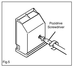
Prise cover loose using screwdriver in position (1) then lever off with screwdriver in position (2) at either side. See Fig. 6.
