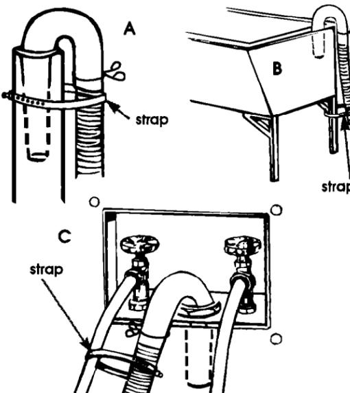
Put "hook" end of drain hose in tub or standpipe. Tightly wrap the shipping strap around the drain hose and tub or standpipe or inlet hose as shown in Figures A-C. Push plug into the nearest hole in the shipping strap.
