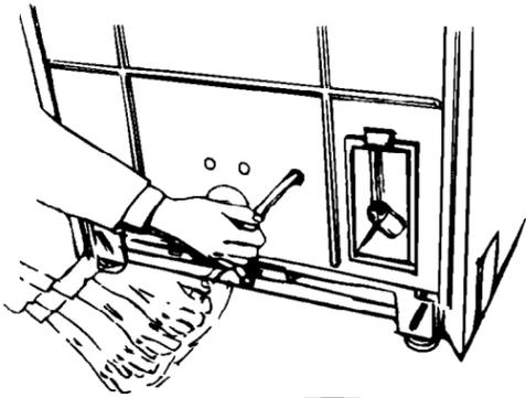
**1.** Pull the strap completely out of the washer.
