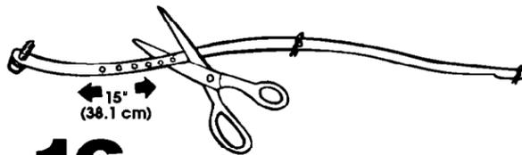
**16.** Measure and mark a point approximately 15 inches (38.1 centimeters) from the plug end of the shipping strap. Cut the shipping strap at this point.
