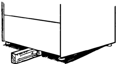
**10.** Carefully tilt washer backwards until front of washer is 3-4 inches (7.5-10 centimeters) off of floor. Insert piece of wood as brace.
