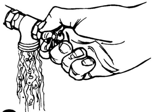
**8.** Before attaching water inlet hose, run water through both faucets into a bucket. This will get rid of particles in the water lines that might clog hoses. Mark which is the hot water faucet.
