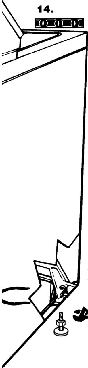
**14.** Tilt washer forward, raising back legs 1 inch (2.5 centimeters) off of floor to adjust rear self-leveling legs. Gently lower washer to floor. Check levelness of the washer by placing a carpenter's level on top of the washer, first side to side; then front to back.
