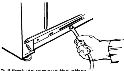
Pull firmly to remove the other end of shipping strap from the back of the washer. The shipping strap plug must be completely removed from the washer for the self-leveling legs to be released.
