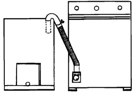
If a longer drain hose is needed, drain hose (Part No. 388423) and hose extension kit (Part No. 285442) are available from authorized parts distributors. If drain hose must be shortened, use hose kit (Part No. 285442).
