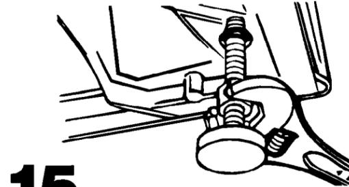
**15.** If washer is not level, screw the front legs up or down to adjust. Repeat Step 14.
