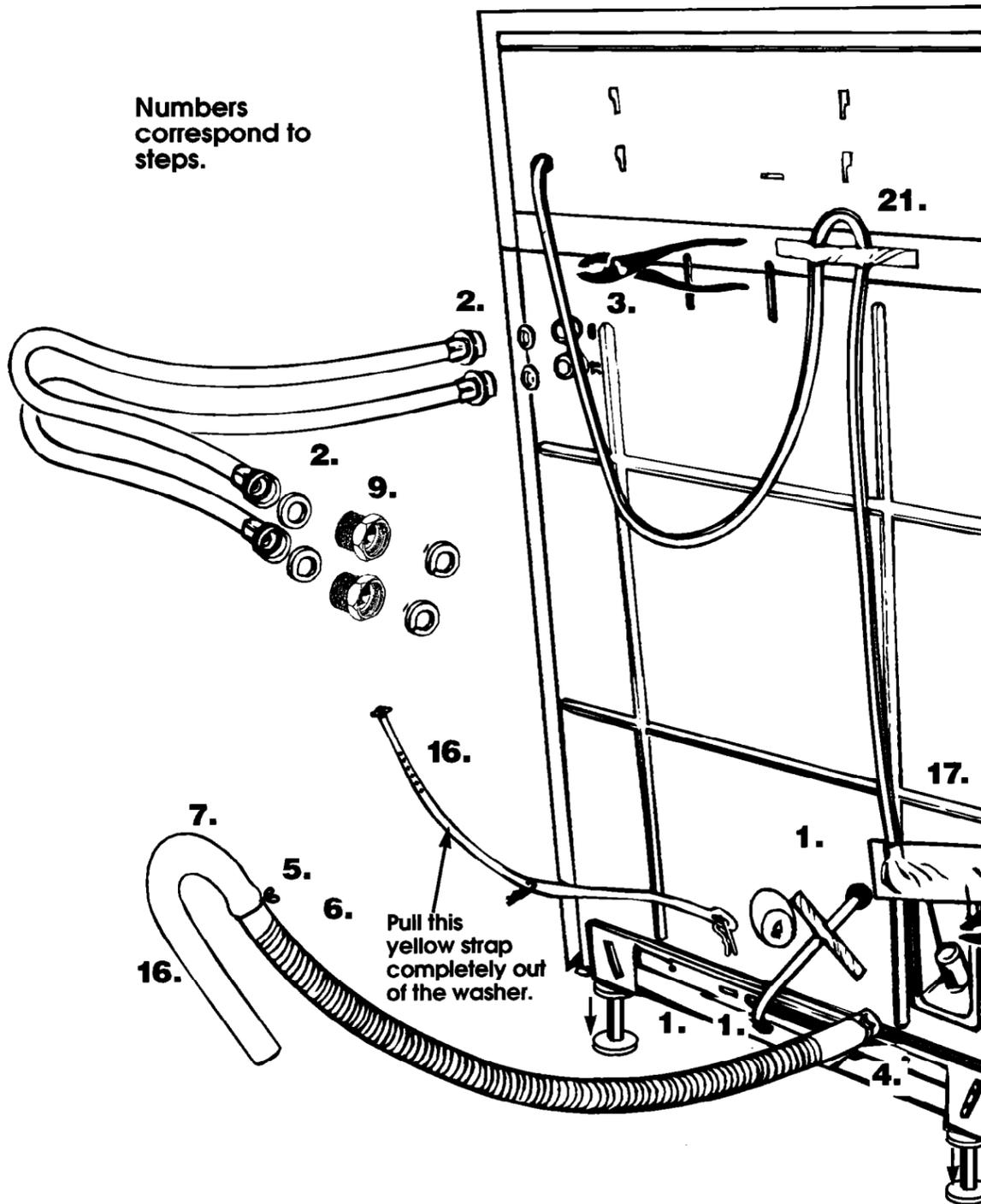
2. Squeeze ears of clamp with pliers to open and place clamp over the end of the drain hose.
