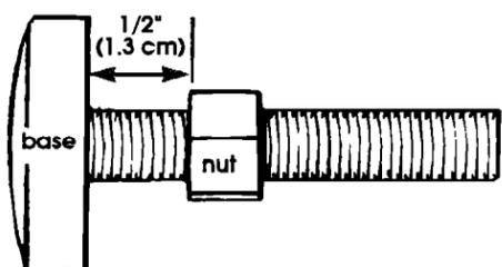
**11.** Use legs and nuts from parts package. Screw nut down to within 1/2 inch (1.3 centimeters) of base.
