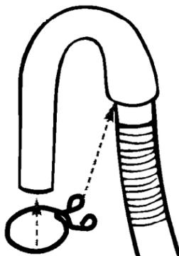
**7.** DO NOT FORCE EXCESS LENGTH OF DRAIN HOSE DOWN THE STANDPIPE. THIS COULD CAUSE SIPHONING.
