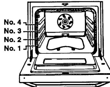
Each oven has three racks. Two racks are straight and the third is offset (raised). The shape of the offset rack helps you space racks better.
