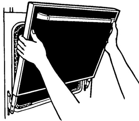
1. **Grasp** door firmly on both sides. **Slide** the hinge slot in the bottom of the door over the hinges. **Push** the door down and in to replace.
