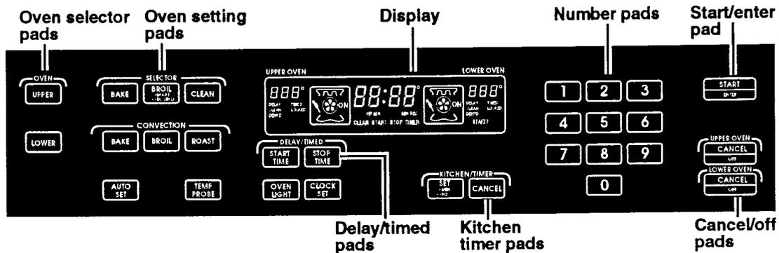
**NOTE:** Examples shown in this Use and Care Guide are for the upper oven only. Lower oven operation is the same; however, the lower oven display is on the right side of the time display.
