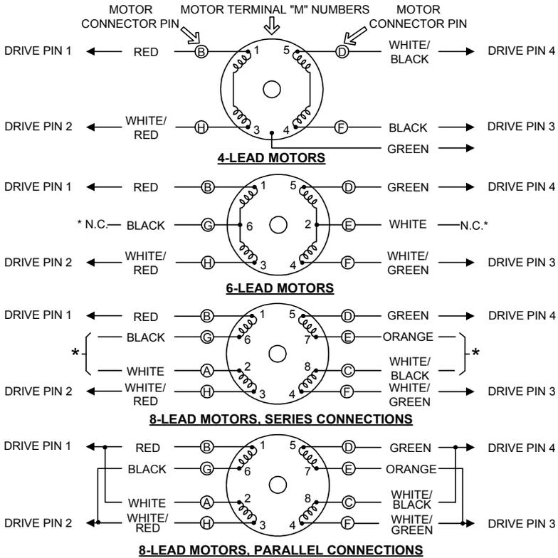
**\*These leads must be insulated and isolated from other leads or ground.**
