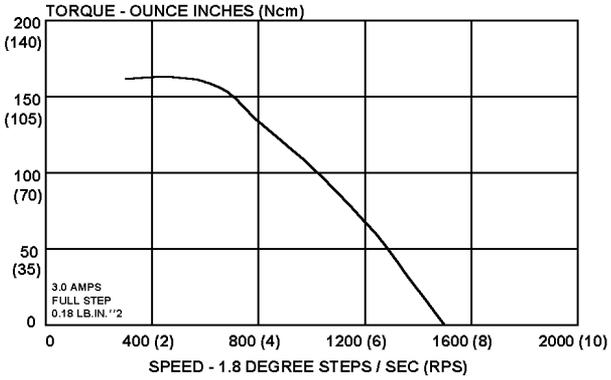
M063-LE09 ETC. MOTORS, SERIES CONNECTED, FULL STEP \*
