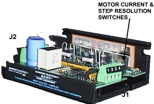
Figure 4.1 Switches For Setting Current Level and Step Resolution
