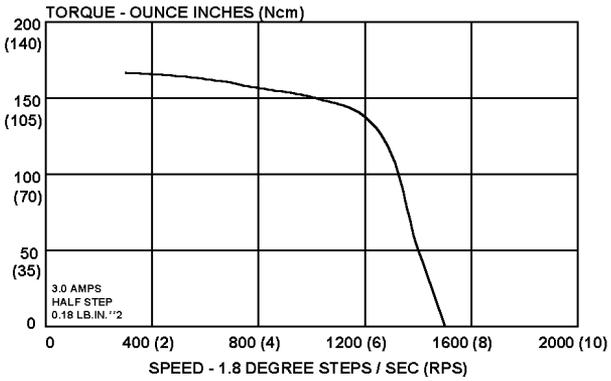
M063-LE09 ETC. MOTORS, SERIES CONNECTED, HALF STEP \*
