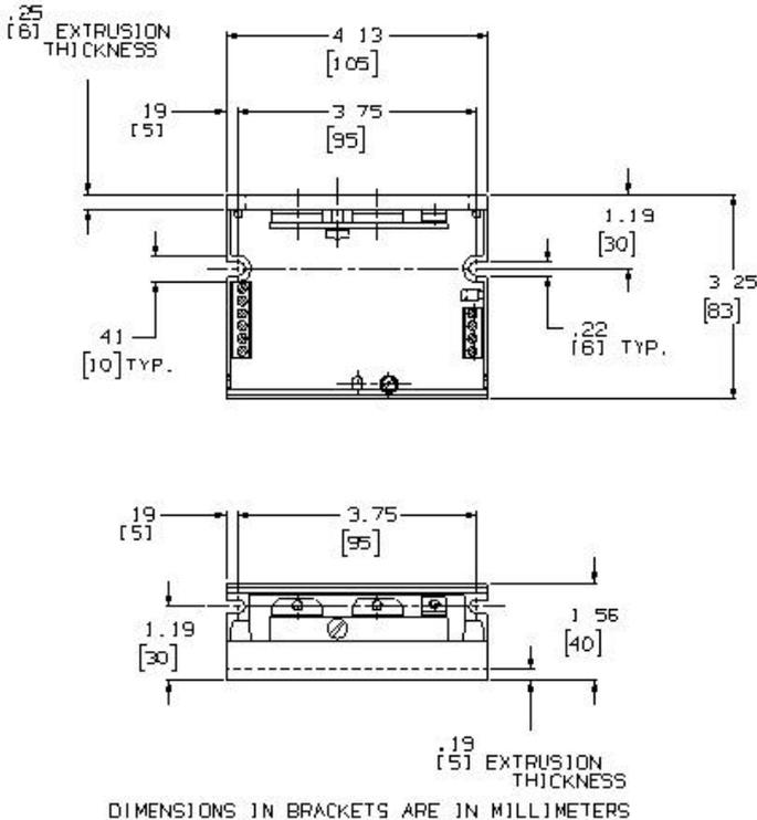
**Figure 3.1 Mounting Diagram**
