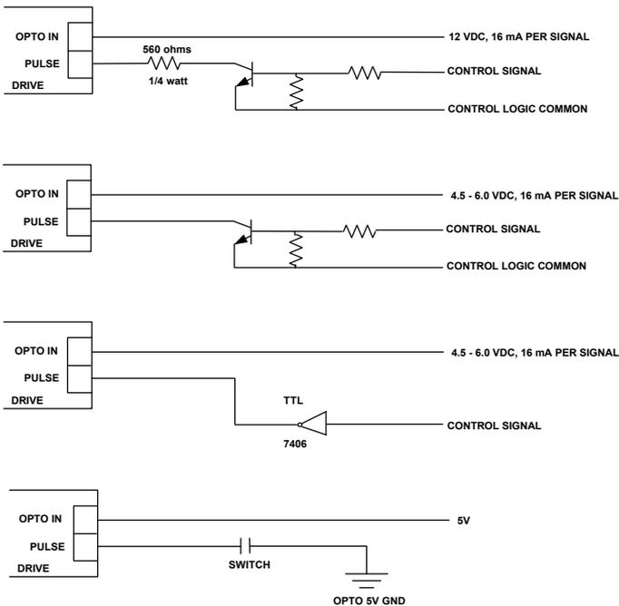
Figure 4.2 Suggested Methods For Control Interface
