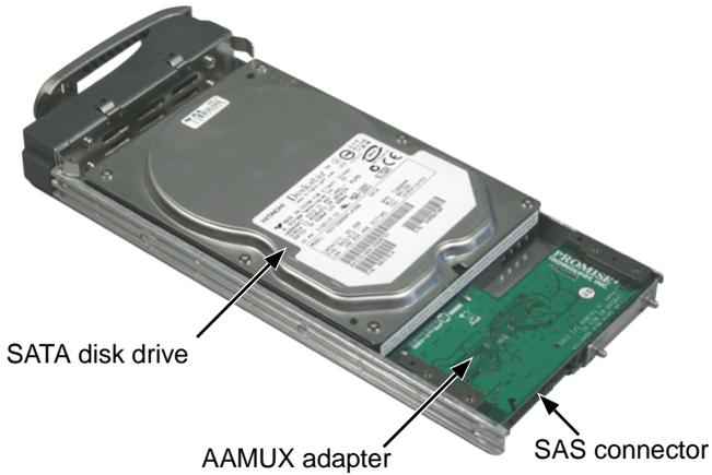
**Figure 9. SAS drive mounted in a drive carrier**
