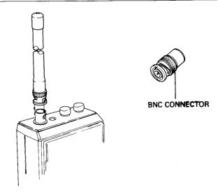
Always use 50 ohm coaxial cable. For length over 50 feet, use RG8 low-loss, dielectric coaxial cable.
