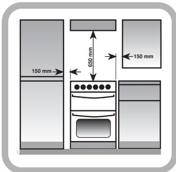
The height of the cooker can be adjusted by means of adjustable feet in the plinth (900mm - 915mm). Adjust the feet by tilting the cooker from the side. Then install the product into position.
