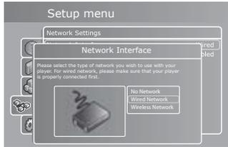
**Network Interface:** Press this menu item to define how your player is connected to your local network. If your player is connected to your hub/switch/router through a cable, select WIRED. If you have a wireless access point and prefer to use this for connection, select WIRELESS.
