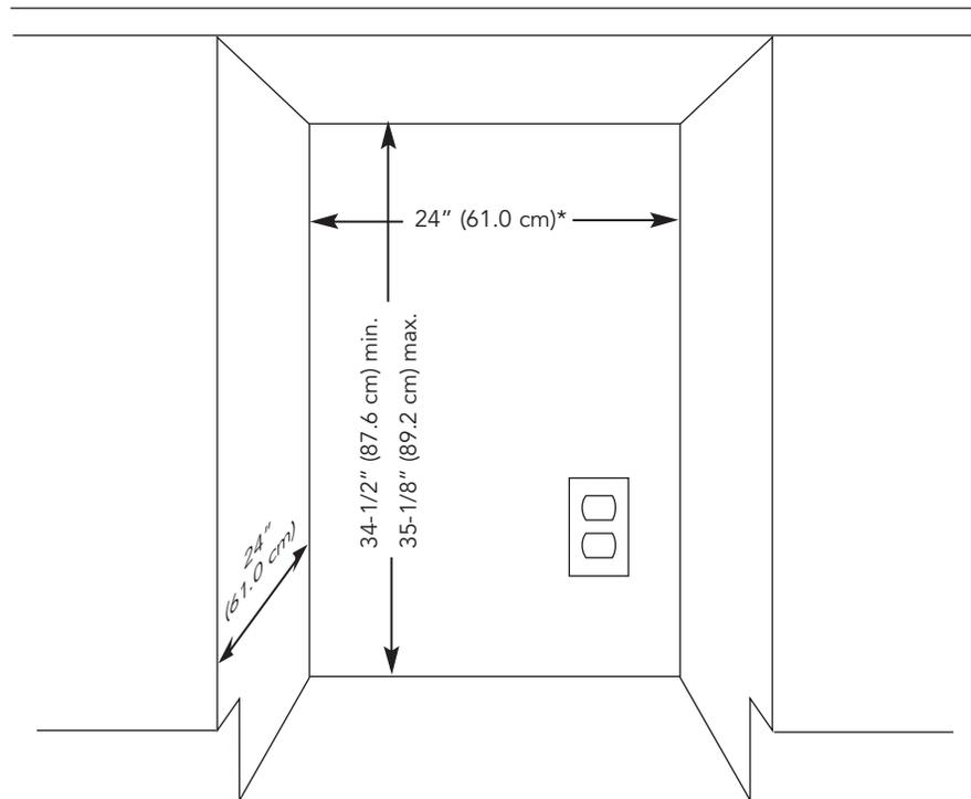
\*Optional: Cutout for electrical outlet can be placed in adjacent cabinetry.
