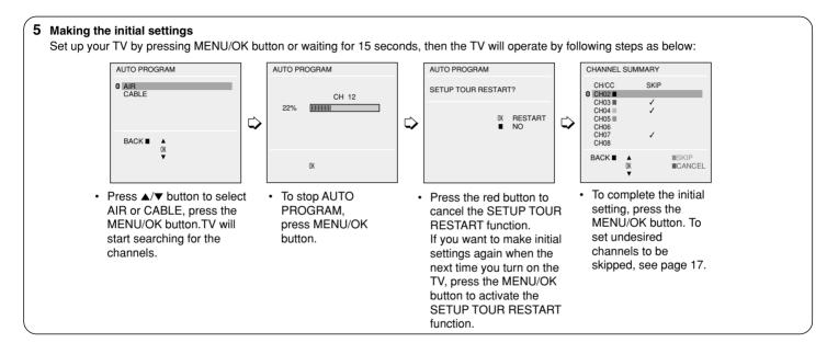
If the JVC logo does not appear, use AUTO PROGRAM function to make the initial settings. This function is located in the INSTALL menu.
