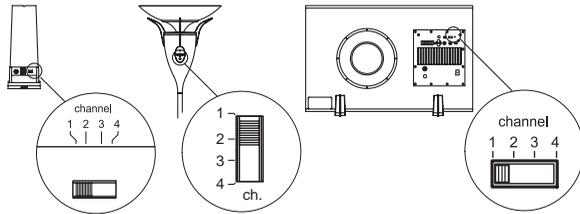
\* if wireless signal interferes with other devices, change both the receiver and the transmitter to different corresponding channels
