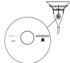
set push button to wireless to receive wireless signal from transmitter
