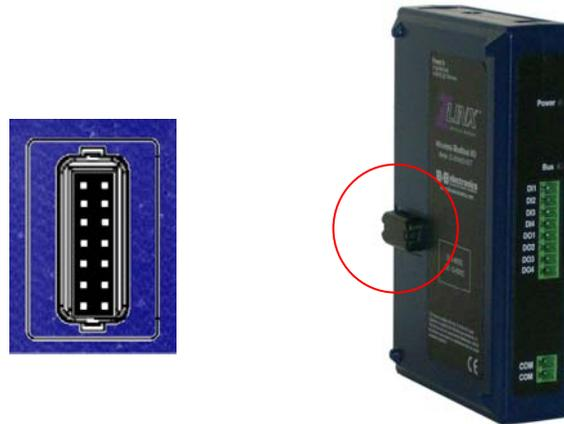
Figure 7. Local Bus Connector Location
