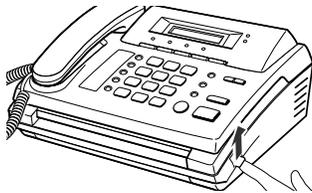
2. Place the paper roll in the compartment so the paper exits from the top of the roll.
