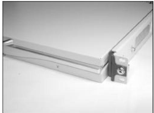
3. Slide the assembled drawer to the rack cabinet from the front and insert the two slide rails of the assembled drawer into the pockets of the rear brackets.
