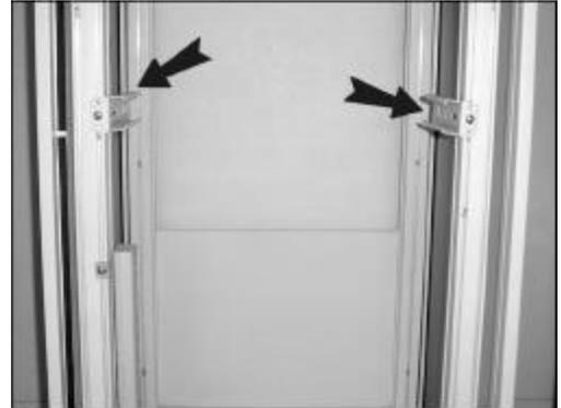
2. Remove the *stopper* from the assembled drawer. The *stopper* is designed to refrain the drawer from sliding out during transportation.
