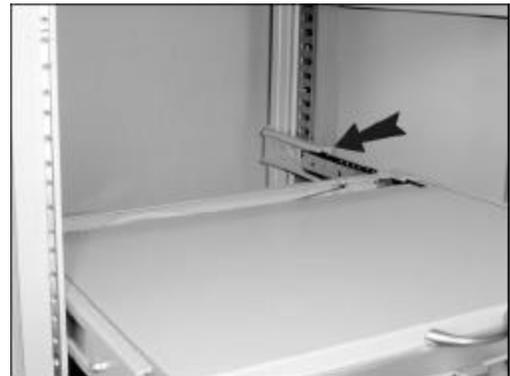
4. Fasten the assembled drawer onto the front brackets by four screws.
