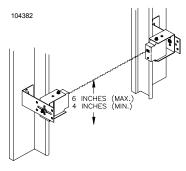
accidental rotation of the bracket NOTE: It is very important that the wall brackets be mounted at exactly the same height so they will be aligned.
