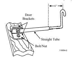
Open and Close limits. Connect curved rod section to trolley.
