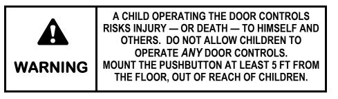
control over the garage door operator and its functions at all times. You may install one Deluxe Wall Station and one or more standard push buttons to a Challenger AC9000 Series operator following the cautions and instructions outlined below.
