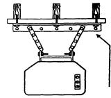
For finished ceilings, or if structural beams are out of position for mounting use a third mounting angle (not included) making sure it is securely mounted to beams.
