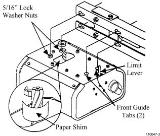
**STEP 5:** The power head drive unit should be move forward until
