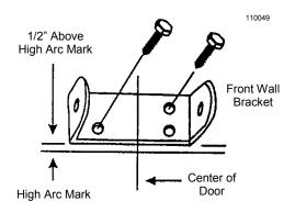
Mount the Front Mounting Bracket securely with lag screws as shown in figure above. If necessary, reinforce the header with steel angle iron or wood to ensure a secure mount.
