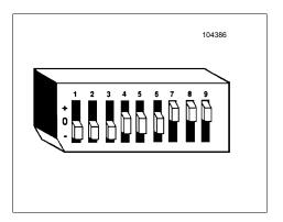
**CODING BLOCK:** Transmitter and Receiver Coding Switches are contained in identical Coding Blocks, consisting of nine small switches, labeled 1 - 9, each of which can be set in any of three positions, labeled +, 0, -
