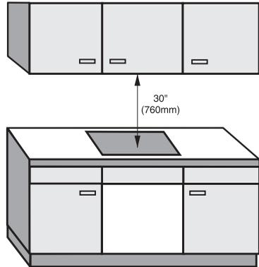
As a general rule there must be a safety distance of at least 30" (760 mm) between the appliance and any objects above it, e.g. cabinetry, venting hood, etc. If the manufacturer of these items states a different figure, always adhere to the greater distance. These measurements should be given in their operating and installation instructions.
